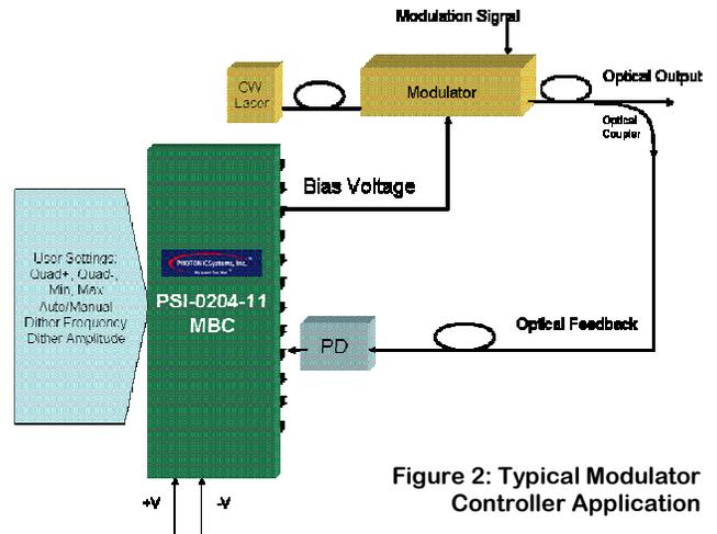
**Figure 2: Typical Modulator Controller Application**
