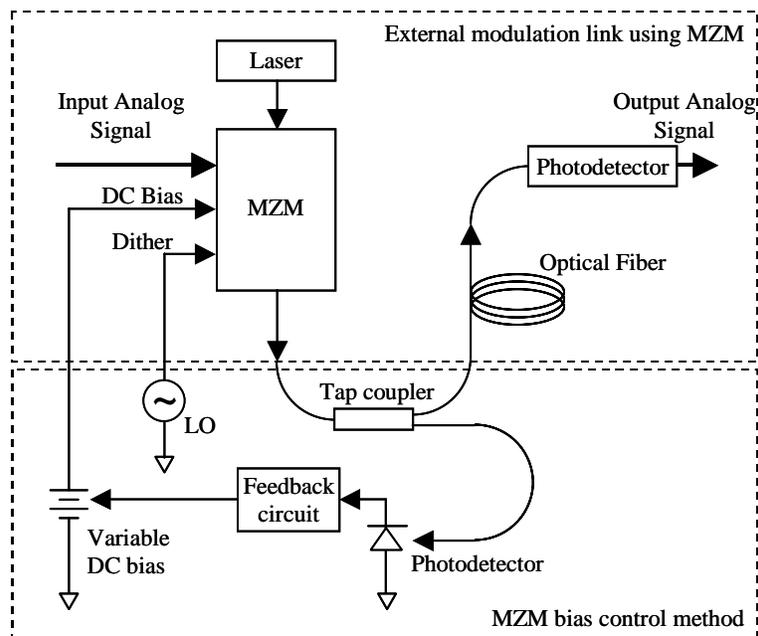
**Figure 8. Method of controlling external modulator bias by injecting a dither signal and using feedback correction to maintain a desired bias point.**
