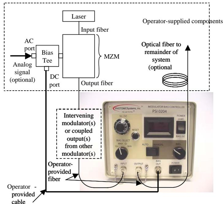
**Figure 5. Required connections for bias control of an MZM with a single electrical input port.**
