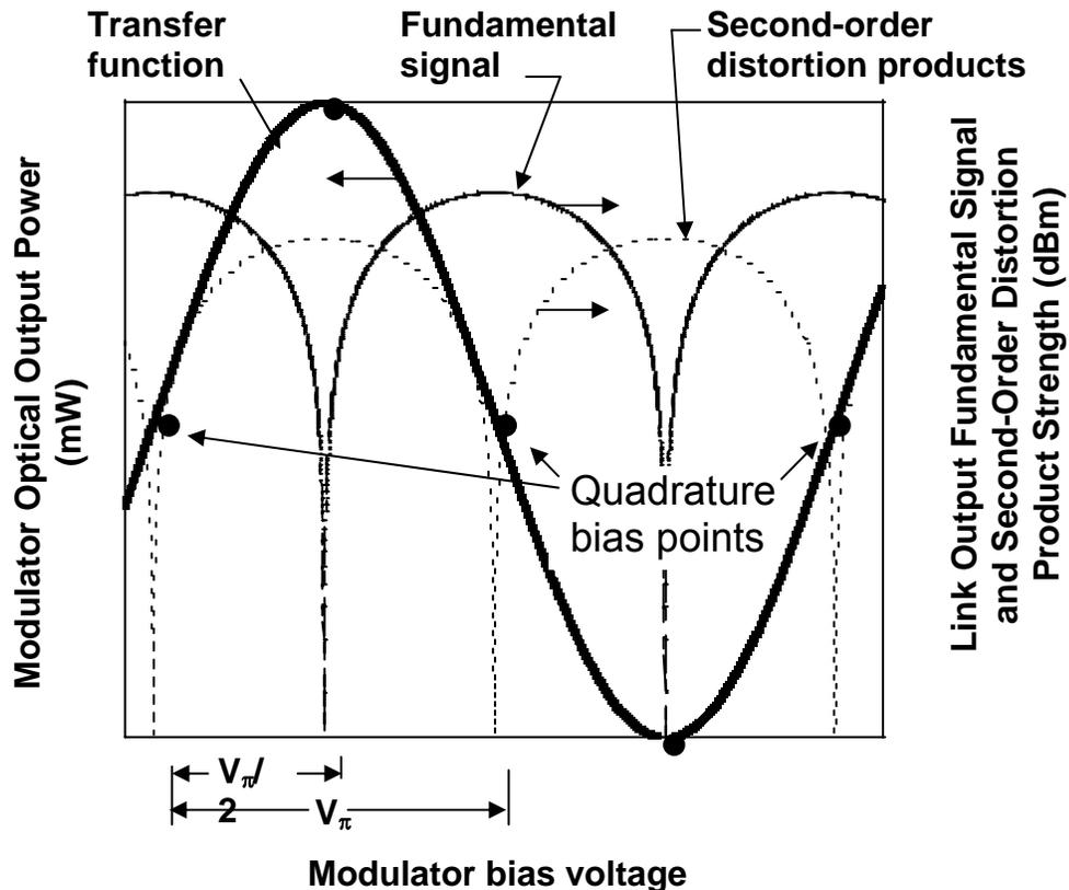
Figure 7. MZM transfer function, and link output power at the fundamental and second-order distortion product frequencies.
