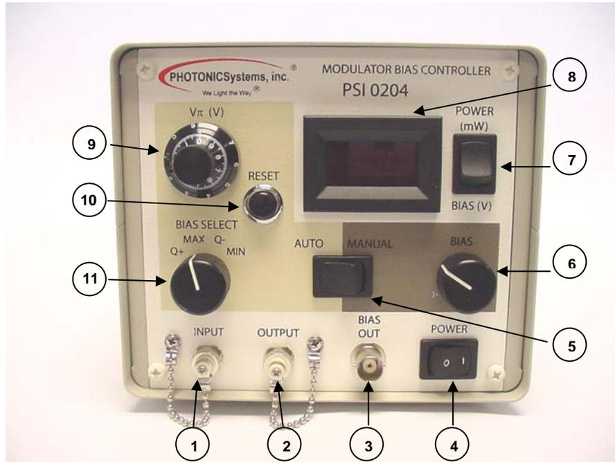
Figure 2. Photograph of the PSI-0204 Modulator Bias Controller with the connections labeled.
