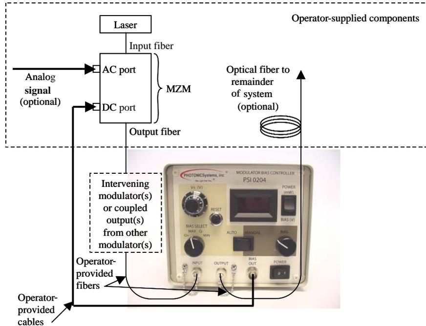
Figure 4. Required connections for bias control of an MZM with separate AC and DC input ports.
