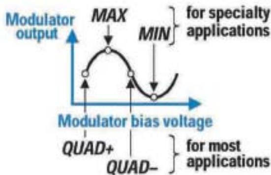
**Figure 1. Modulator Transfer Function**
