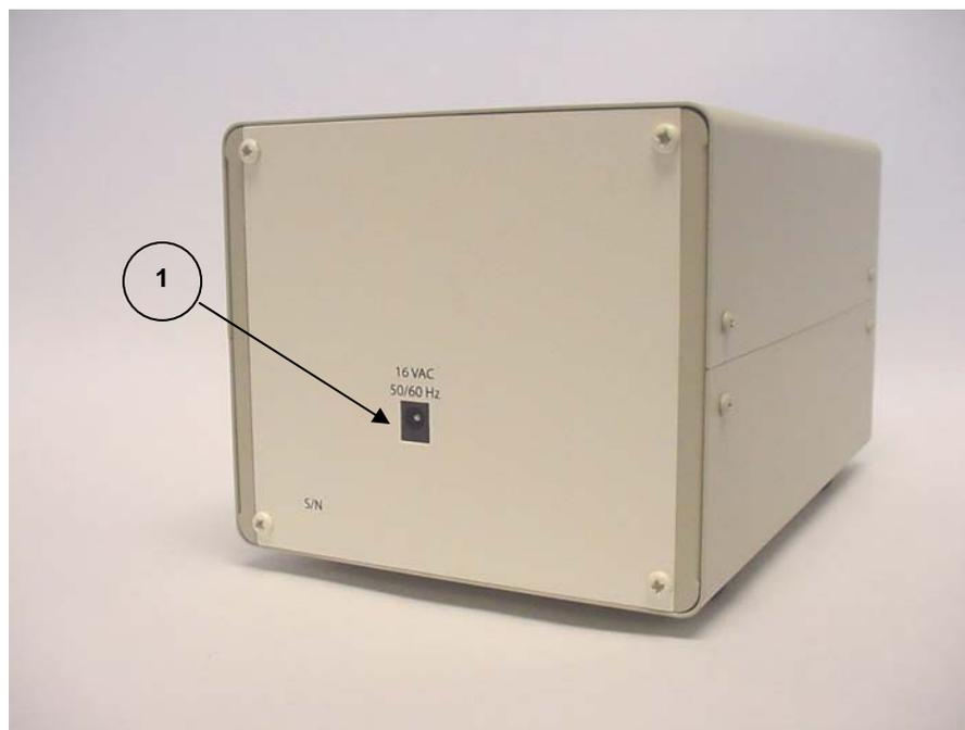
**Figure 3. Photograph of the rear panel of the PSI-0204 Modulator Bias Controller with the connection labeled.**
